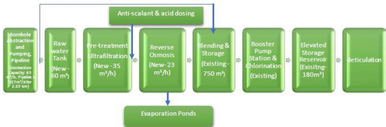
Figure 6: Desalination process train at Bethanie
