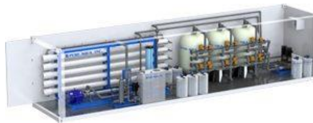
Figure 3: Containerized reverse osmosis desalination system
